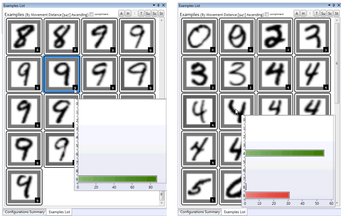
Figure 5.2: Prospect allows programmers to see the distribution of predicted labels for each example. Here the nine on the right is correctly classified by all of the configurations, the four on the right is misclassified some of the time. In some configurations it is classified as a nine. This information would be impossible to see by looking at the results for any given model.
